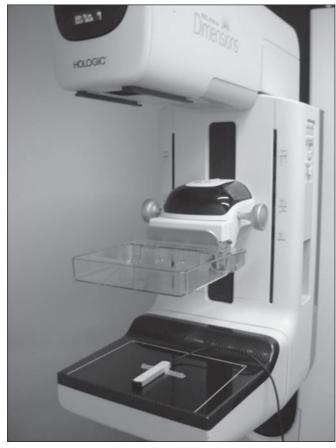
Figure 2. Solid-state detector positioning for measurement of Ki and HVL.
