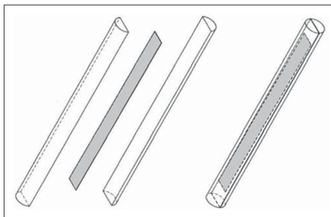
**Figure 2.** Positioning of the radiochromic film in the PMMA cylinder.
