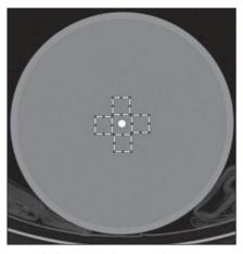
Figure 3. CT section of phantom for quality study, with four selected central areas selected in the ImageJ software for image noise calculation.
