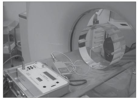
Figure 1. Electrometer, ionization chamber and body phantom exposed to the tomographic beam for CTDI calculation.
