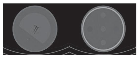
Figure 4. CT sections of phantom for quality study and analysis of image spatial resolution and contrast.
